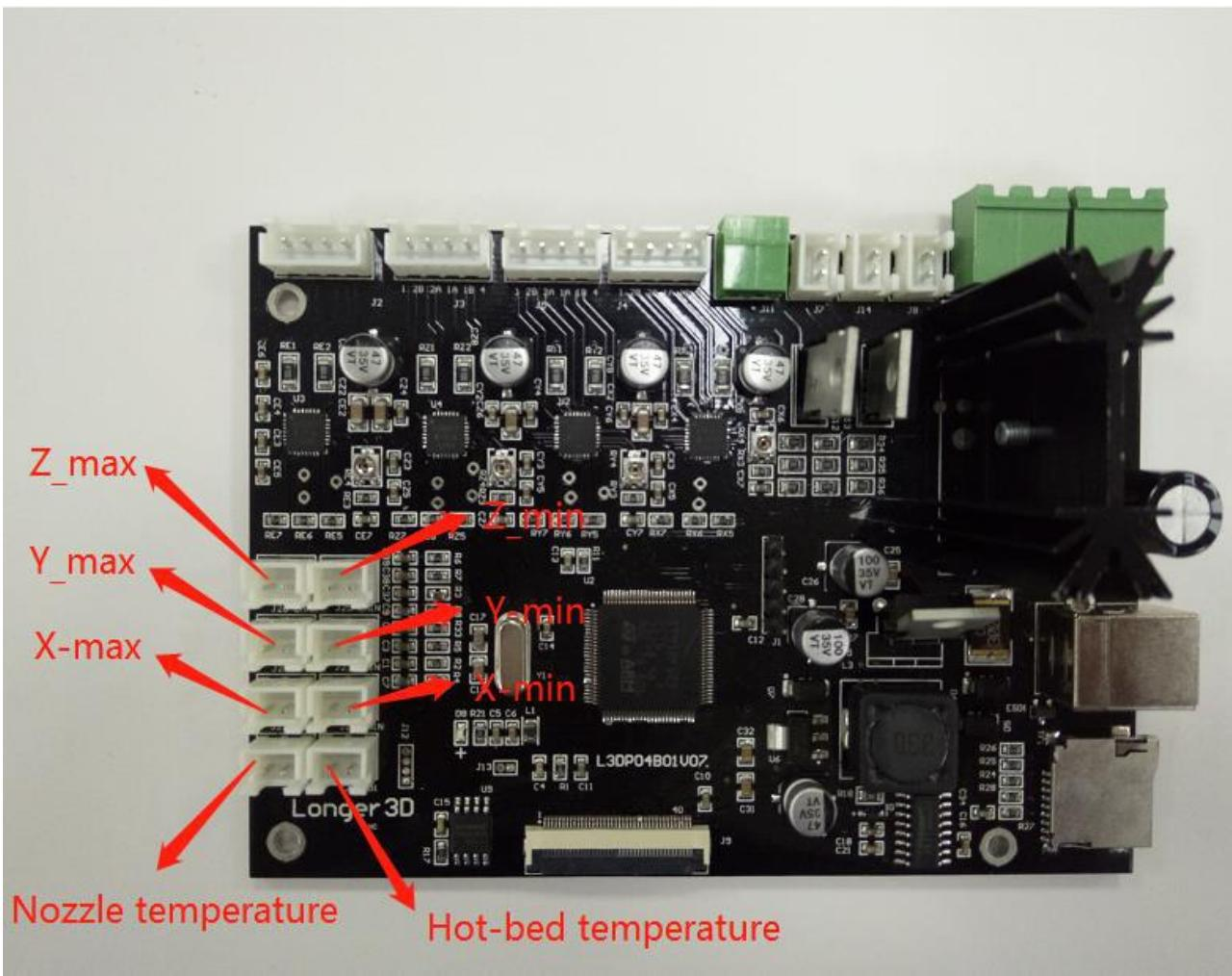
The current function of X\_max is filament run-out detection(E-).
